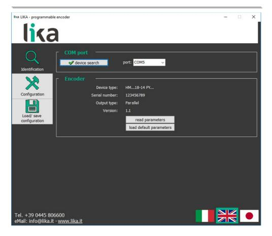
Should this happen, please check the unit is connected properly and the power is on. Make sure that the power supply voltage is correct. Also check that the serial cable characteristics meet the requirements described in the "4.11 RS-232 serial connection" section on page 22.
