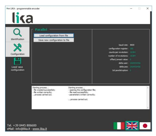
This page allows the operator to save the current encoder configuration to a .dat file; or to load a previously saved configuration. The current encoder configuration is listed in the pane on the right.
